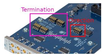
Figure 3: Position of switches
